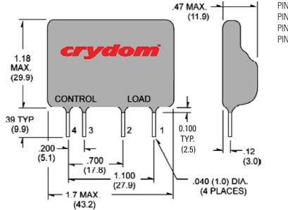
PIN 1: AC LOAD PIN 2: AC LOAD PIN 3: +DC CONTROL PIN 4: -DC CONTROL THERMAL DERATE INFORMATION
